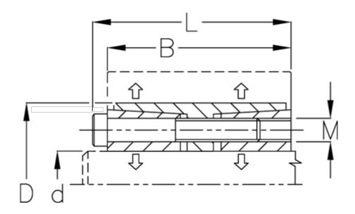
B mm = 54d H8 mm = 42D mm = 75Fit tolerance = Aksel h8, Nav H8
